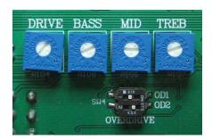
**Boost Preamp** – Drive, Bass, Midrange and Treble internal trimpots to customize your Overdrive level and tone. The dip switch is used to select OD1 (Normal) Boost or OD2 (Super Boost) Overdrive. Note: Only one OD switch can be selected at a time or the overdrive circuitry will oscillate.
