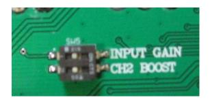
The Input Gain dip switch adds +10dB of gain to the first stage input buffer. This adds more drive to both channels. The Ch2 Boost switch adds a +20dB Mid/Treble boost to the clean channel for more tube like growl.
