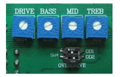
**Boost Preamp** – Drive, Bass, Midrange and Treble internal trimpots to customize your Overdrive level and tone. The dip switch is used to select OD1 (Normal) Boost or OD2 (Super Boost) Overdrive. Note: Only one OD switch can be selected at a time or the overdrive circuitry will oscillate.
