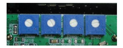
**Boost Preamp EQ** – Controls are accessable thru the bottom cover. The internal Bass, Midrange, Mid Frequency and Treble trimpots can be used to customize your Boost Overdrive tone.
